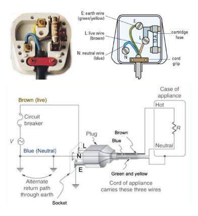
• A fused plug is used to connect appliances to the mains supply via the power socket.
