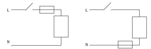
A fault in the appliance leads to a short circuit causing the current to increase. This melts the fuse and opens the circuit and the appliance stops working. (in the case of a circuit breaker, it trips and opens the circuit)
