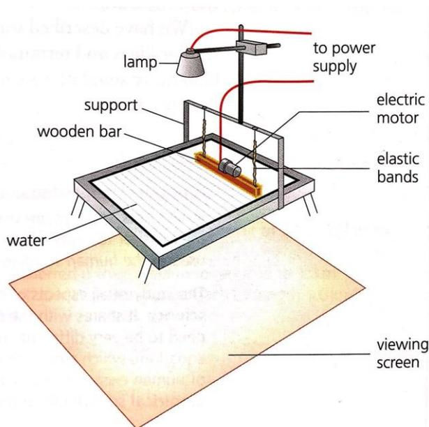
Waves on a ripple tank are produced continuously by a motor that vibrates a small dipper or beam suspended on the water surface. It can be used to study wave behavior.
